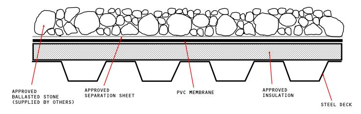
APPROVED INSULATION: UL CLASSIFIED POLYISOCYANURATE INSULATION.
