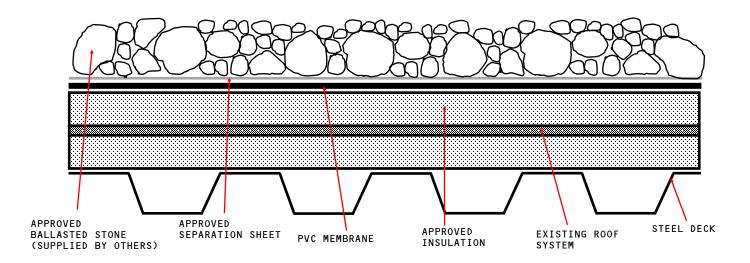
APPROVED INSULATION: UL CLASSIFIED POLYISOCYANURATE INSULATION.
