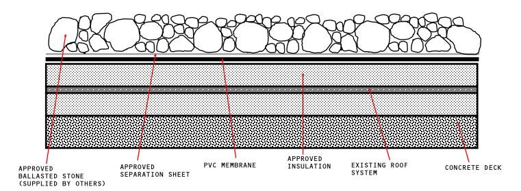
APPROVED INSULATION: UL CLASSIFIED POLYISOCYANURATE INSULATION.
