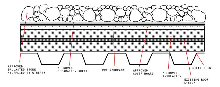
APPROVED COVER BOARD: DENS DECK, DENS DECK PRIME OR SECUROCK GLASS-MAT, MINIMUM 1/4" THICKNESS.
