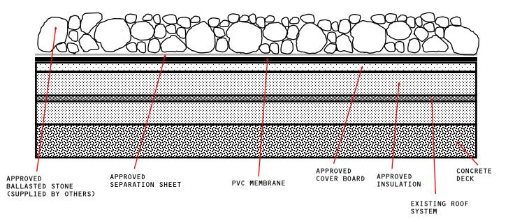
APPROVED COVER BOARD: DENS DECK, DENS DECK PRIME OR SECUROCK GLASS-MAT, MINIMUM 1/4" THICKNESS. APPROVED INSULATION: UL CLASSIFIED POLYISOCYANURATE, EXPANDED POLYSTYRENE, EXTRUDED POLYSTYRENE INSULATION.
