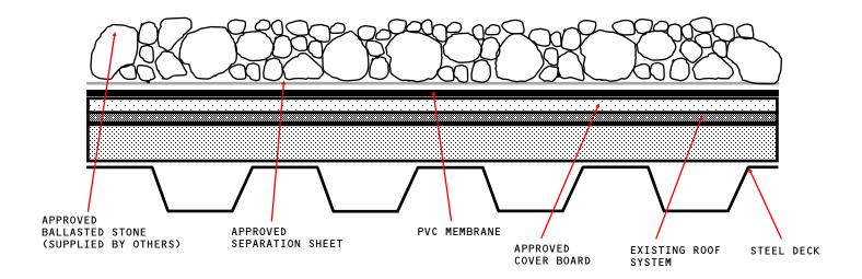
APPROVED COVER BOARD: DENS DECK, DENS DECK PRIME OR SECUROCK GLASS-MAT, MINIMUM 1/4" THICKNESS. APPROVED SEPARATION SHEET: 4 OZ OR 6 OZ GEOTEXTILE SEPARATION SHEET.
