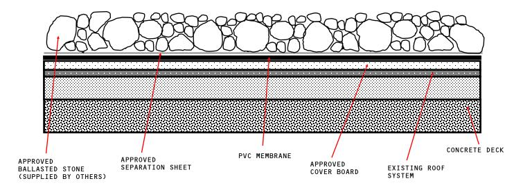
APPROVED COVER BOARD: DENS DECK, DENS DECK PRIME OR SECUROCK GLASS-MAT, MINIMUM 1/4" THICKNESS. APPROVED SEPARATION SHEET: 4 OZ OR 6 OZ GEOTEXTILE SEPARATION SHEET.
