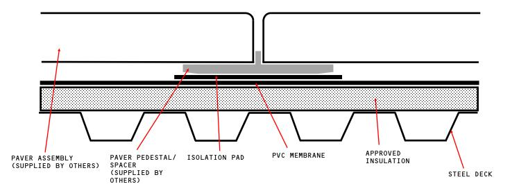
APPROVED INSULATION: UL CLASSIFIED POLYISOCYANURATE INSULATION.
