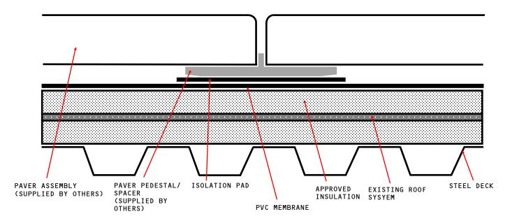
APPROVED INSULATION: UL CLASSIFIED POLYISOCYANURATE INSULATION.
