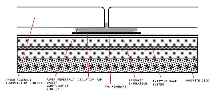
APPROVED INSULATION: UL CLASSIFIED POLYISOCYANURATE INSULATION.
