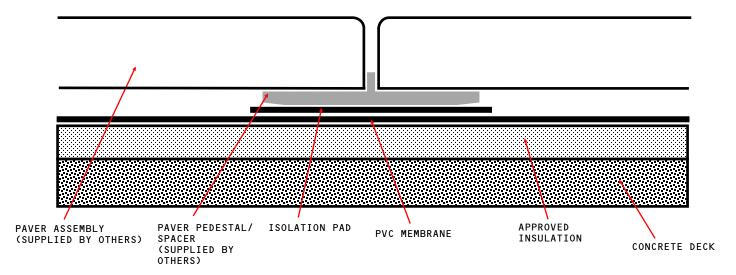
APPROVED INSULATION: UL CLASSIFIED POLYISOCYANURATE INSULATION.
