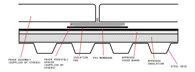
APPROVED COVER BOARD: DENS DECK, DENS DECK PRIME OR SECUROCK GLASS-MAT, MINIMUM 1/4" THICKNESS. APPROVED INSULATION: UL CLASSIFIED POLYISOCYANURATE, EXPANDED POLYSTYRENE, EXTRUDED POLYSTYRENE INSULATION.
