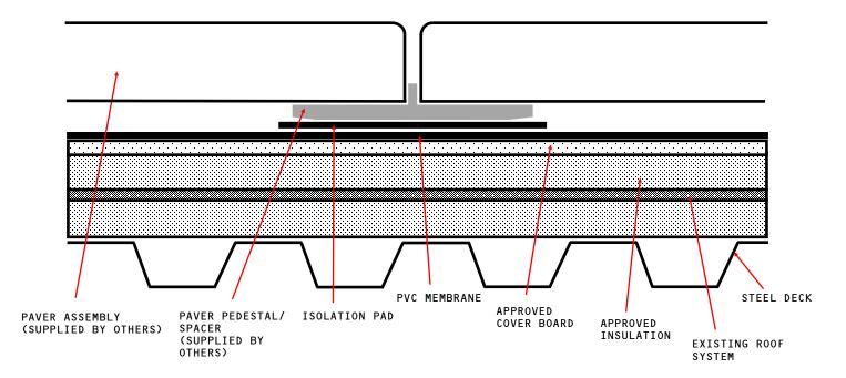
APPROVED COVER BOARD: DENS DECK, DENS DECK PRIME OR SECUROCK GLASS-MAT, MINIMUM 1/4" THICKNESS. APPROVED INSULATION: UL CLASSIFIED POLYISOCYANURATE, EXPANDED POLYSTYRENE, EXTRUDED POLYSTYRENE INSULATION.
