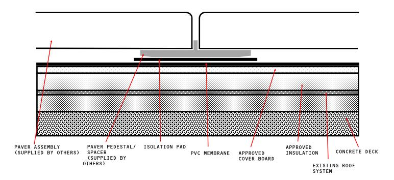
APPROVED COVER BOARD: DENS DECK, DENS DECK PRIME OR SECUROCK GLASS-MAT, MINIMUM 1/4" THICKNESS.
