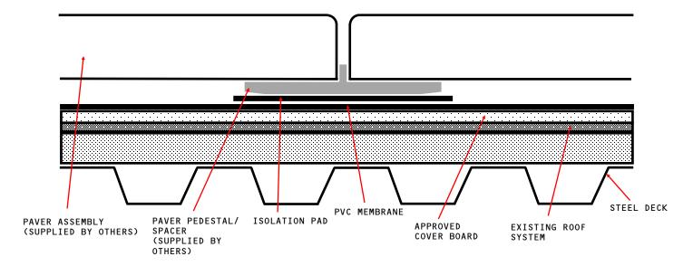
APPROVED COVER BOARD: DENS DECK, DENS DECK PRIME OR SECUROCK GLASS-MAT, MINIMUM 1/4" THICKNESS.
