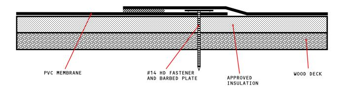
APPROVED INSULATION: UL CLASSIFIED POLYISOCYANURATE INSULATION.
