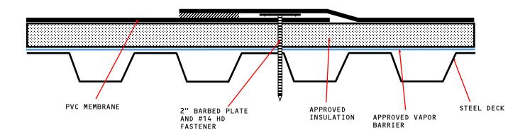
APPROVED INSULATION: UL CLASSIFIED POLYISOCYANURATE INSULATION.
