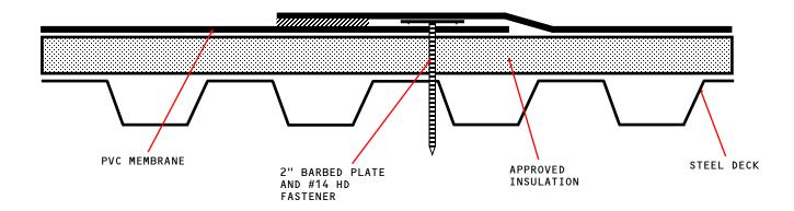
APPROVED INSULATION: UL CLASSIFIED POLYISOCYANURATE INSULATION.
