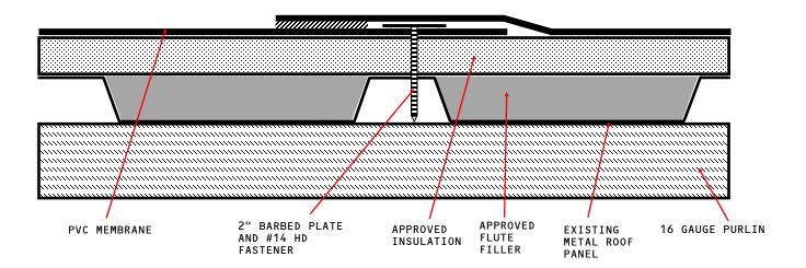
APPROVED INSULATION: UL CLASSIFIED POLYISOCYANURATE INSULATION.
