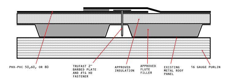
APPROVED INSULATION: HUNTER PANELS, RMAX OR ATLAS UL CLASSIFIED INSULATION.
