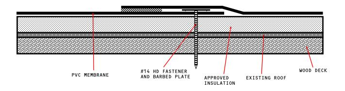
APPROVED INSULATION: UL CLASSIFIED POLYISOCYANURATE INSULATION.
