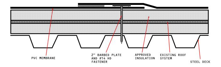
APPROVED INSULATION: UL CLASSIFIED POLYISOCYANURATE INSULATION.
