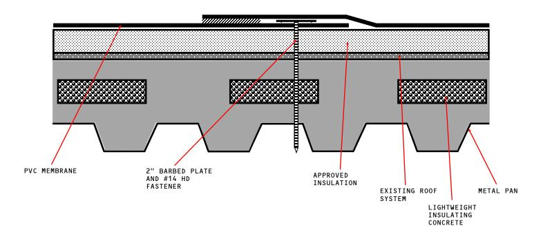
APPROVED INSULATION: UL CLASSIFIED POLYISOCYANURATE INSULATION.
