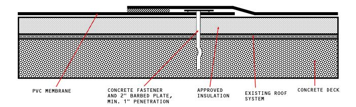
APPROVED INSULATION: UL CLASSIFIED POLYISOCYANURATE INSULATION.
