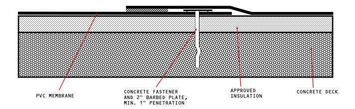
APPROVED INSULATION: UL CLASSIFIED POLYISOCYANURATE INSULATION.
