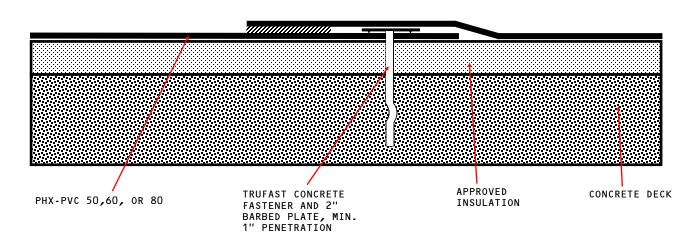
APPROVED INSULATION: HUNTER PANELS, RMAX OR ATLAS UL CLASSIFIED INSULATION.
