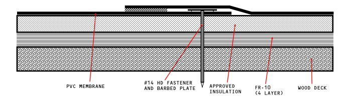
APPROVED INSULATION: UL CLASSIFIED POLYISOCYANURATE INSULATION TYPE II AND III.
