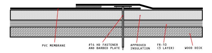
APPROVED INSULATION: UL CLASSIFIED POLYISOCYANURATE INSULATION TYPE II AND III.
