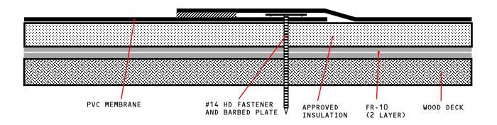
APPROVED INSULATION: UL CLASSIFIED POLYISOCYANURATE INSULATION TYPE II AND III.
