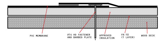
APPROVED INSULATION: UL CLASSIFIED POLYISOCYANURATE INSULATION.
