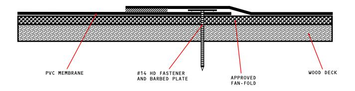
APPROVED INSULATION: Any UL Classified Expanded and Extruded Polystyrene Fanfold min 1.5 lb density and minimum 1/2" thick.
