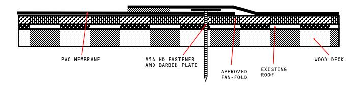
APPROVED INSULATION: Any UL Classified Expanded and Extruded Polystyrene Fanfold min 1.5 lb density and minimum 1/2" thick.
