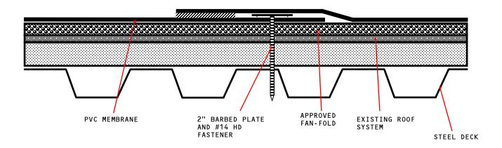
APPROVED INSULATION: Any UL Classified Expanded and Extruded Polystyrene Fanfold min 1.5 lb density and minimum 1/2" thick.
