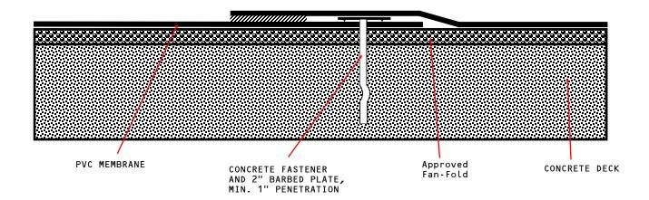
APPROVED INSULATION: Any UL Classified Expanded and Extruded Polystyrene Fanfold min 1.5 lb density and minimum 1/2" thick.
