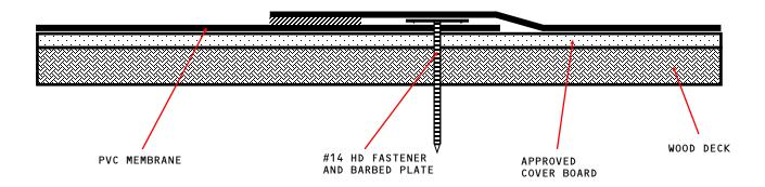
APPROVED COVER BOARD: DENS DECK, DENS DECK PRIME OR SECUROCK GLASS-MAT, MINIMUM 1/4" THICKNESS.
