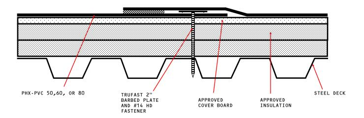
APPROVED COVER BOARD: DENS DECK, MINIMUM 1/4" THICKNESS. APPROVED INSULATION: HUNTER PANELS, RMAX OR ATLAS UL CLASSIFIED INSULATION.
