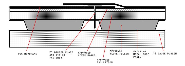
APPROVED COVER BOARD: DENS DECK, DENS DECK PRIME OR SECUROCK GLASS-MAT, MINIMUM 1/4" THICKNESS.
