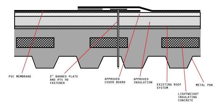
APPROVED COVER BOARD: DENS DECK, DENS DECK PRIME OR SECUROCK GLASS-MAT, MINIMUM 1/4" THICKNESS.
