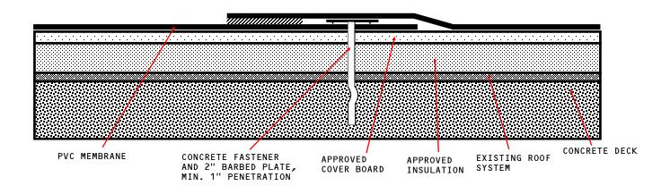
APPROVED COVER BOARD: DENS DECK, DENS DECK PRIME OR SECUROCK GLASS-MAT, MINIMUM 1/4" THICKNESS. APPROVED INSULATION: UL CLASSIFIED POLYISOCYANURATE, EXPANDED POLYSTYRENE, EXTRUDED POLYSTYRENE INSULATION.
