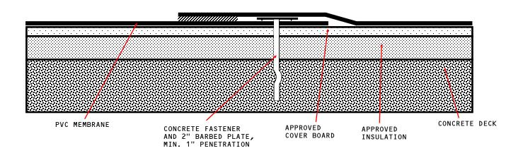
APPROVED COVER BOARD: DENS DECK, DENS DECK PRIME OR SECUROCK GLASS-MAT, MINIMUM 1/4" THICKNESS. APPROVED INSULATION: UL CLASSIFIED POLYISOCYANURATE, EXPANDED POLYSTYRENE, EXTRUDED POLYSTYRENE INSULATION.
