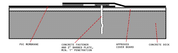
APPROVED COVER BOARD: DENS DECK, DENS DECK PRIME OR SECUROCK GLASS-MAT, MINIMUM 1/4" THICKNESS.
