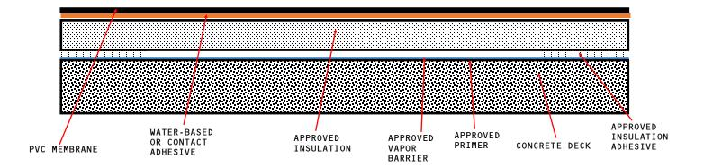
APPROVED INSULATION: UL CLASSIFIED POLYISOCYANURATE INSULATION.
