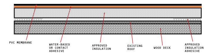
APPROVED INSULATION: UL CLASSIFIED POLYISOCYANURATE INSULATION.
