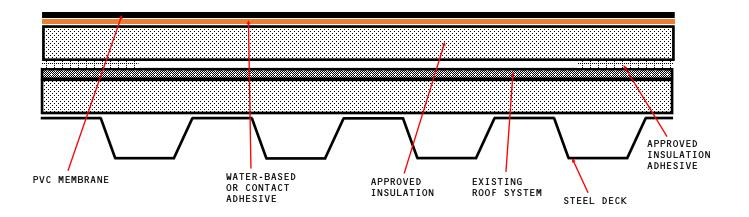
APPROVED INSULATION: UL CLASSIFIED POLYISOCYANURATE INSULATION.
