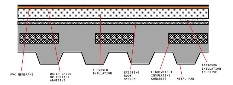
APPROVED INSULATION: UL CLASSIFIED POLYISOCYANURATE INSULATION.
