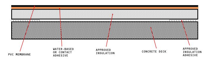
APPROVED INSULATION: UL CLASSIFIED POLYISOCYANURATE INSULATION.
