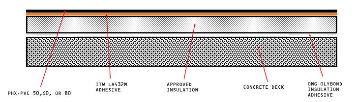
APPROVED INSULATION: HUNTER PANELS, RMAX OR ATLAS UL CLASSIFIED INSULATION.
