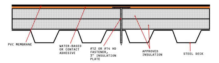
APPROVED INSULATION: UL CLASSIFIED POLYISOCYANURATE INSULATION.
