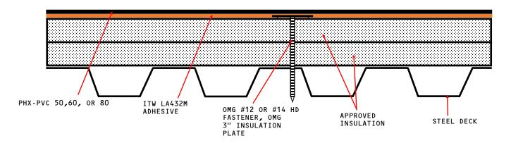
APPROVED INSULATION: HUNTER PANELS OR ATLAS UL CLASSIFIED INSULATION.
