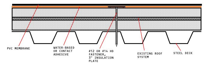
APPROVED INSULATION: UL CLASSIFIED POLYISOCYANURATE INSULATION.
